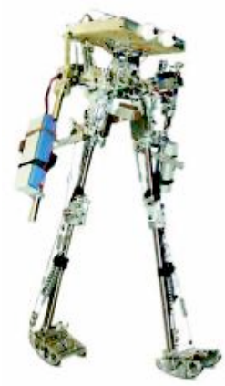
From left to right: Delft, MIT, and Cornell walking robots. The Cornell biped weighs about 13 kg and dissipates roughly 11 W total. To
